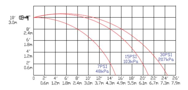
K5.6 STANDARD HORIZONTAL SIDEWALL DISTRIBUTION PATTERNS – PLAN VIEW
